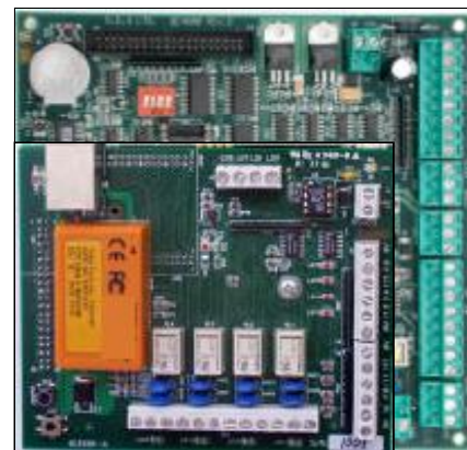
Toplock 4 D4 ZD controller PCB with TCP/IP and RS485
