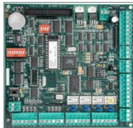
Toplock 3 D3 ZD controller PCB
